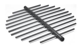
**SWT's Water's Edge Header Systems** are custom fabricated from noncorrosive FDA and NSF approved materials. For use in softeners, carbon filters, multimedia filters, and waste water applications, they are available for tanks from 48 to 120 inches in diameter and are optimized for your application—whether you need 3.5 or 20 gpm/sq.ft.
